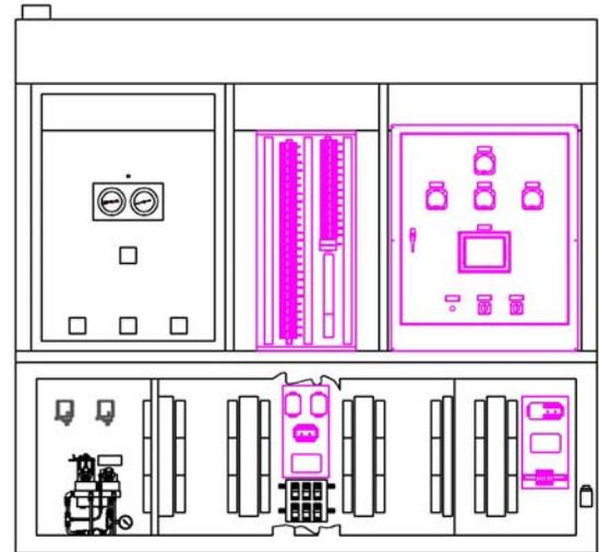
Figure 15: Installation Arrangement of New Governor Panels in Actuator Cabinet
