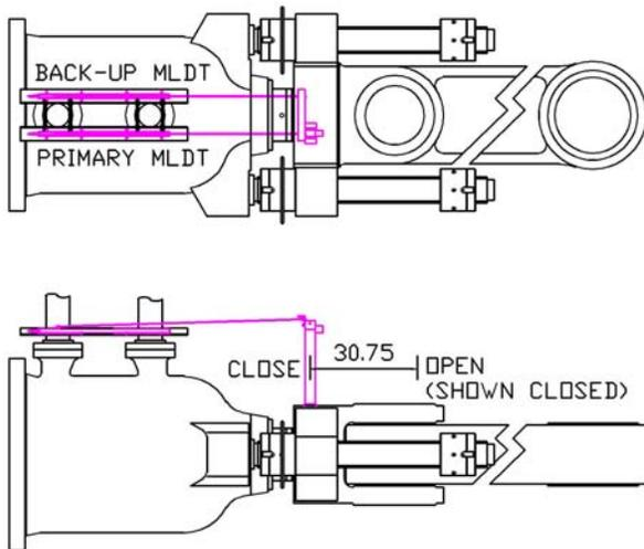
Figure 16: Installation Arrangement of Primary and Back-up MLDTs
