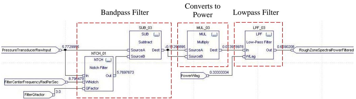
Figure 5: Block diagram of Rough Zone Detection Filter
