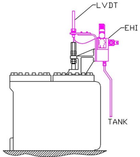
Figure 17: Installation Arrangement of Electro-hydraulic Interface
