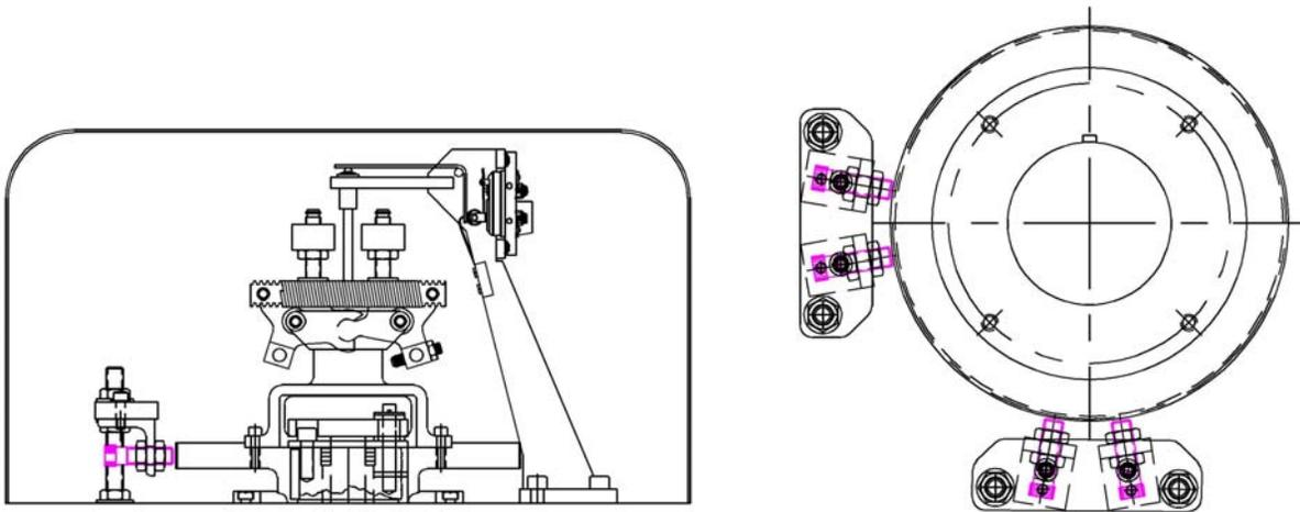
Figure 9: Proximity Sensors Used for Governor Speed and Creep Detection
