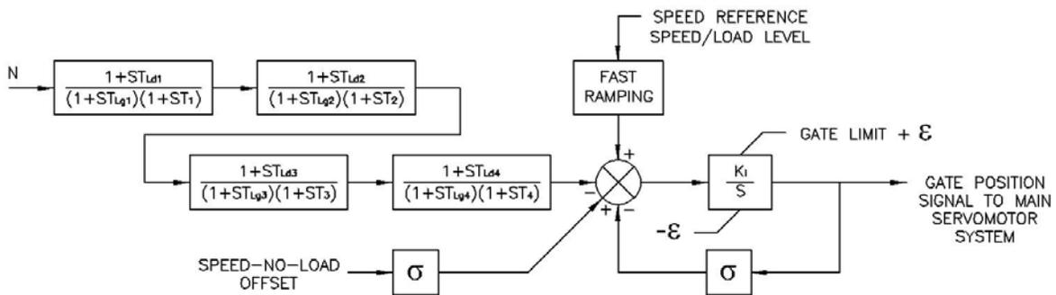
Figure 8: USBR Four-Stage Lead-Lag Algorithm
