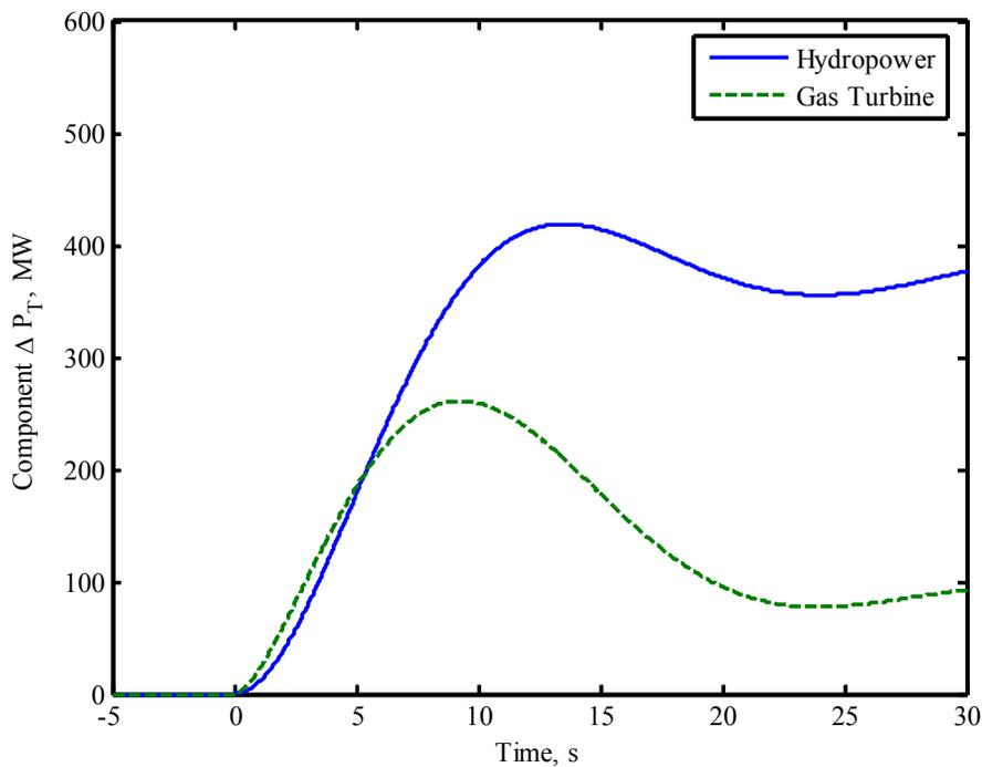
**Figure 10: Power Contribution from Hydropower and Gas Turbines after a Power Generation Dropout of 500 MW on WECC,  $X=33\%$**
