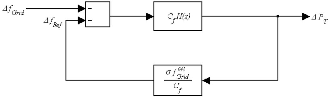
**Figure 5: General linearized turbine model**
