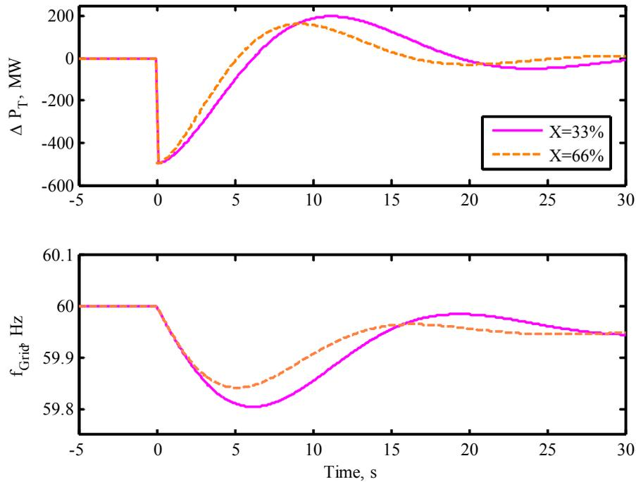
**Figure 8: Simulated Turbine Power and Frequency Response after a Power Generation Dropout of 500 MW on WECC,  $X=33\%$  and  $X=66\%$**
