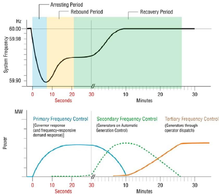
Figure 2: Sequence of Dominant Action by Primary, Secondary, and Tertiary Frequency response. Source: (Eto, et al., 2010)
