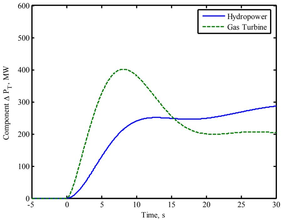
**Figure 12: Power Contribution from Hydropower and Gas Turbines after a Power Generation Dropout of 500 MW on WECC,  $X = 66\%$**
