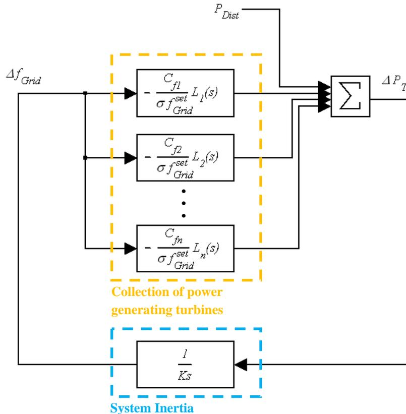
**Figure 7: Linearized model for a collection of power generating turbines subject to small frequency and load changes.**
